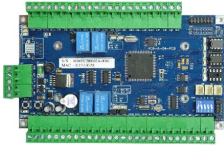
Serial Lift Access Control Panel (L3800)
