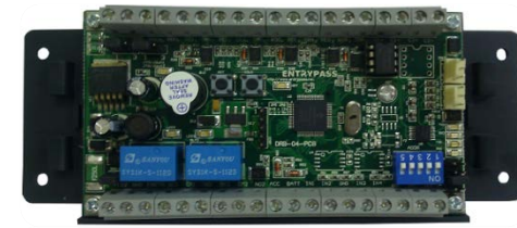
Networked Integrated Reader Controller (N-MINI 2 – N618, N668)
